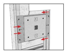
5. Cut and install the drywall around the fixture, ensuring that the fixture board assembly is flush with the surrounding drywall. This will allow a finish of one eight inch of plaster around the finishing guard.
