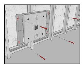
1. Fasten the bracket to the framing in the desired fixture location. Insure that the "TOP" label is facing towards the ceiling and the "DOWN" label is facing towards the floor.
