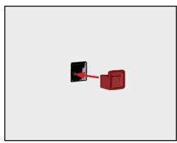
10. Carefully remove the finishing guard from the fixture opening. Then, insert the louver into the fixture opening to magnetically attach the louver.
