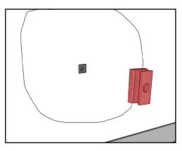
8. Wait until the surface has fully dried, and sand the plastered ceiling to match the surrounding level of drywall.
