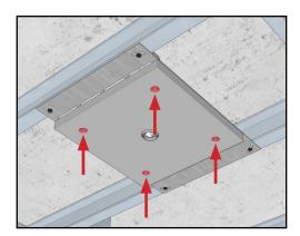
5. Secure the board to the drywall bracket using the provided screws.
