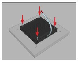
3. Take the Minus fixture and place it onto the mounting board. Secure the Minus fixture to the board by fastening the screws provided with the fixture.
