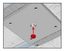
7. Insert the finishing guard into the fixture opening to prepare for finishing. The fixture must remain off for the remainder of the installation. The fixture will be damaged if turned on with the finishing guard inserted.
