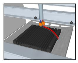
4. Feed low voltage wiring to the bracket and lift the fixture board assembly to the low voltage electrical connection and make the connection.
