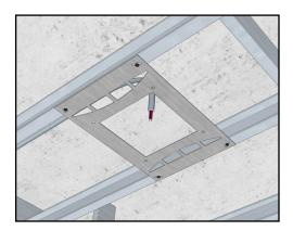
1. Separate the mounting bracket and mounting board and fasten the bracket to the framing in the desired fixture location.
