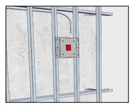
1. Identify the desired fixture location and raise the bracket to the framing.
