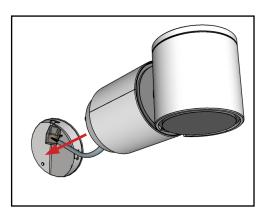
13. Make the low voltage electrical connection.
